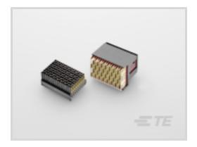
Connector System: Board-to-Board Number of Positions: 112 Row-to-Row Spacing: 1.35 mm [.053 in ] Mating Alignment: With Mating Alignment Type: Keyed
