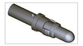
Contact Type: Pin D-Sub Contact Size: 8 Contact Base Material: Copper Alloy Contact Mating Area Plating Material: Gold Termination Method to Wire & Cable: Crimp
