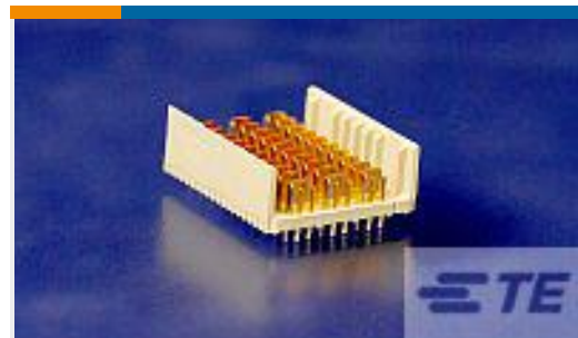
TE Part #2170245-1 HMZD+,3PAIRS,10COLS,VERTICAL, ASSEMBLY
