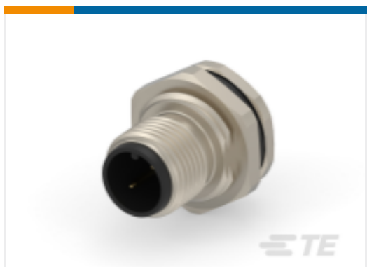
TE Part #T4171010002-001 M12,REAR MOUNTING,MALE,A,2P,0.2 M WIRE
