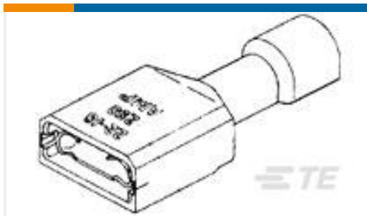
TE Part #2-520405-2 ULTRA-FAST 250 ASY REC 22-18 TPBR
