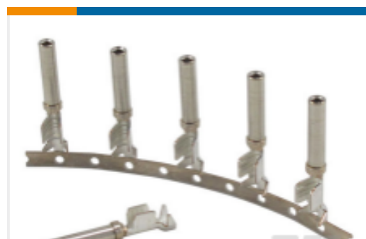
TE Part #2098253-1 SOC, SF, SIZE 16, 14-16 AWG, AU/SN
