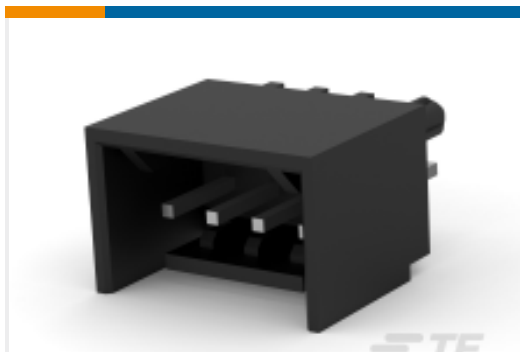
TE Part #2-644486-2 Polyester Vertical PCB Header: 2.54 mm, Shrouded, MTA 100
