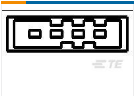
TE Part #1-1903328-4 DYNAMIC 4200S HDR ASSY H 4P X
