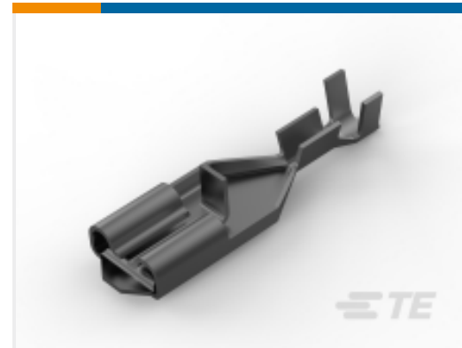
TE Part # 170327-1 250 PL MKII REC. 22-18AWG PTBR
