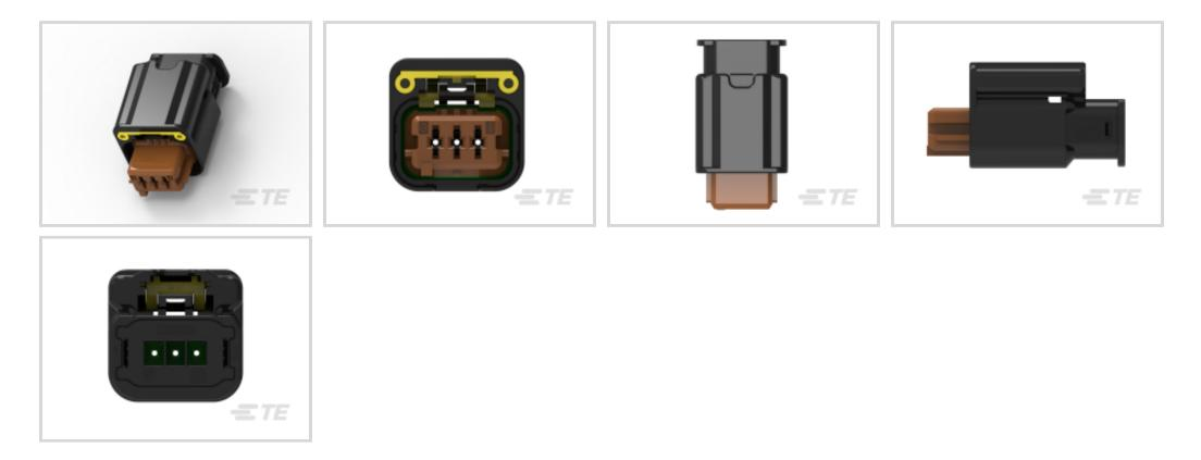
Connector & Housing Type: Housing for Female Terminals Mating Tab Width: .64 mm, 1.5 mm [ .025 in, .059 in ] Connector System: Wire-to-Wire Number of Positions: 3 Centerline (Pitch): 3.33 mm [ .131 in ]
