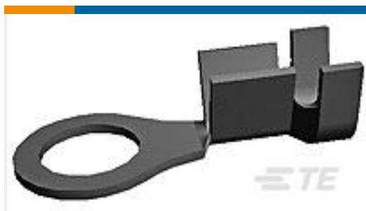
TE Part #42037-1 RING TERMINAL 22-18 AWG TPBR
