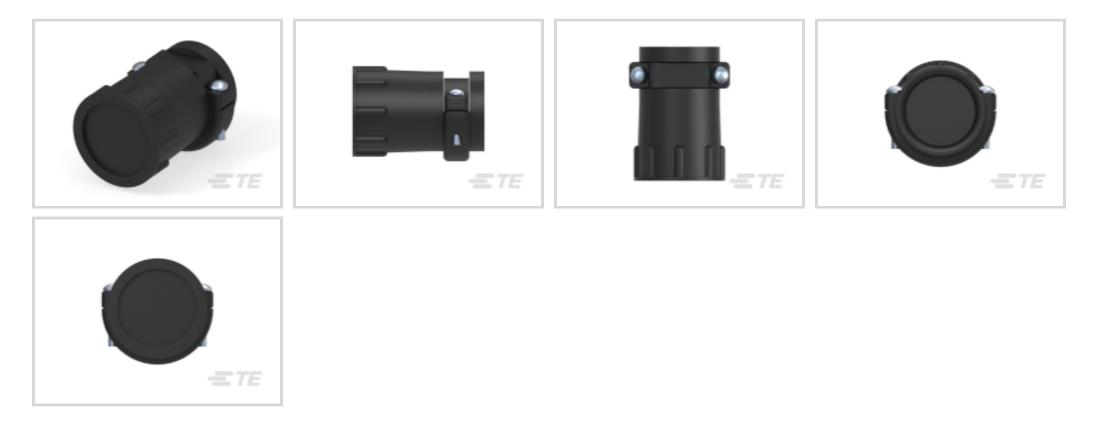
Backshell & Clamp Accessory Type: Cable Clamp Compatible With Circular Connector Shell Size: 17 Body Orientation: Straight Accepts Cable Diameter (Max): 17.86 mm [.703 in ] Protective Cover: Without
