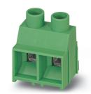
PCB terminal block, nominal current: 32 A, rated voltage (III/2): 1000 V, nominal cross section: 4 mm², Number of potentials: 2, Number of rows: 1, Number of positions per row: 2, product range: MKDSV 5 HV, pitch: 9.52 mm, connection method: Screw connection with tension sleeve, mounting: Wave soldering, conductor/PCB connection direction: 0 °, color: green, Pin layout: Linear back pinning, Solder pin [P]: 5.2 mm, type of packaging: packed in cardboard
