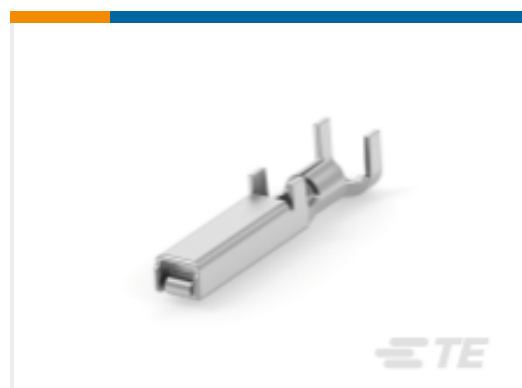
TE Part #353718-5 Contact: Component To Wire; 15A, 28-14 wire size
