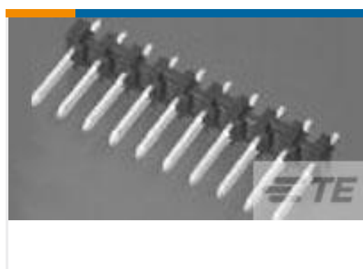
TE Part #827872-9 9P MOD1 UNSHRD HDR, P 5.08, ST, 0.8 Au
