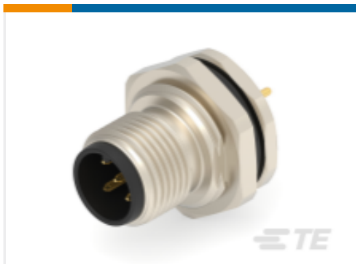
TE Part #T4140012051-000 M12,REAR MOUNTING,MALE,A CODE,5P
