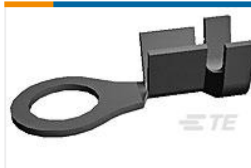
TE Part #160344-2 RING TONGUE 20-16 AWG .025 X .840
