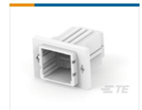
TE Part #2-917809-2 Receptacle and Tab Housing: 5.08 or 10.16 mm pitch, 250-600V
