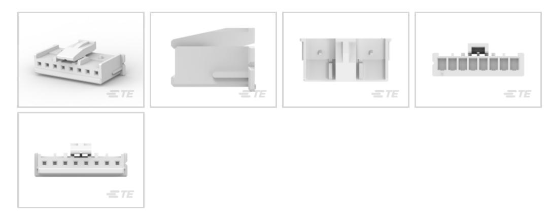
Connector Product Type: Housing Connector & Housing Type: Receptacle Connector System: Wire-to-Board Number of Positions: 8 Centerline (Pitch): 2.5 mm [.098 in ]
