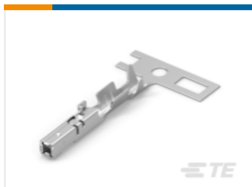
TE Part #1674311-7 0.64 III RCPT 3 Serrations Pre-Tin
