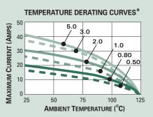
\*The test data are based on single circuits in free space and were generated using a "Lumped Resistance" model. This model does not account for all of the variables that would be present in an actual application. For actual product performance, contact your regional support representative at the number listed below.
