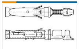
TE Part #163088-2 LOOSE PC SOCKET TYPEIII+ CONTACT SIZE16
