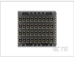
Connector System: Board-to-Board
