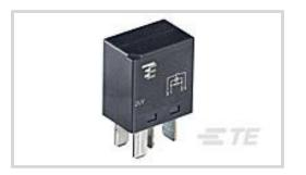
Rated Coil Voltage: 12 VDC Micro Relay Contact Current Class: 20 – 30 A Micro Relay Contact Arrangement: 1 Form A (NO) Micro Relay Coil Resistance: 119  $\Omega$ Mounting Brackets: Without
