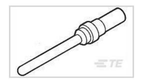
Contact Type: Pin D-Sub Contact Size: 20 Contact Base Material: Brass Contact Mating Area Plating Material: Gold Termination Method to Wire & Cable: Crimp
