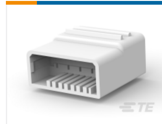
TE Part # 9-144836-5 DOUBLE LOCKING 5 MM HOUSING TAB PA66
