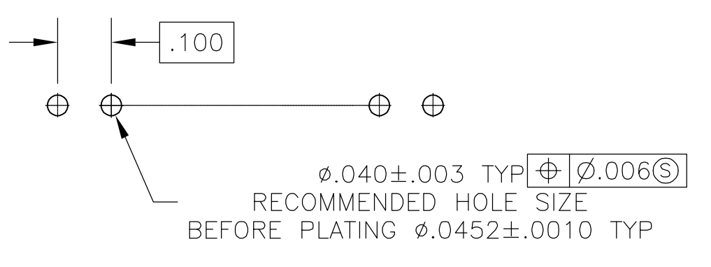
RECOMMENDED HOLE LAYOUT
