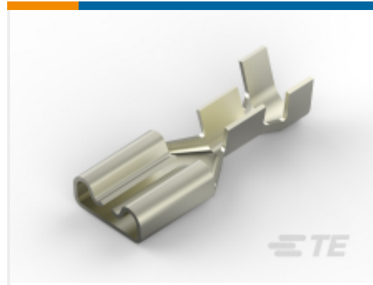
TE Part # 1742198-1 250 FASTON,REC.,18-14 AWG,NPST
