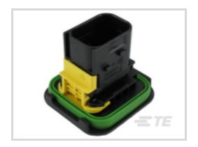
Connector & Housing Type: Housing for Male Terminals Mating Tab Width: 1.6 mm, 2.8 mm [.063 in, .11 in ] Connector System: Wire-to-Wire Number of Positions: 7 Centerline (Pitch): 4 mm, 6 mm [.157 in, .236 in ]
