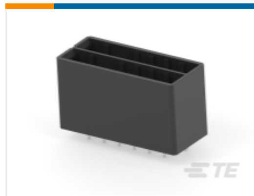
TE Part #2-316132-3 Header Assembly: Wire-to-Board, 15A, gold or tin plated
