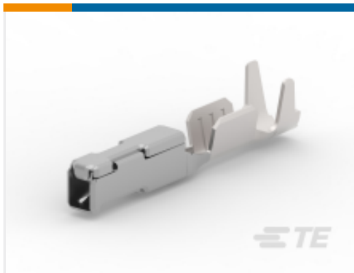
TE Part #1456968-3 CONTACT,FEMALE, 0.64, 20 TO 22 AWG, AG
