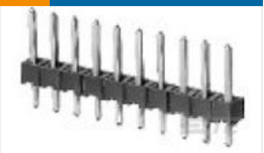
TE Part #5-146277-5 05 MODII HDR SRST B/A .100CL
