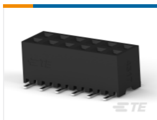
TE Part #1-2314846-4 14P, 2MM, BB, REC, DRVT, SMD, AU.76, TB, W/CP
