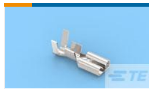
TE Part #881624-2 187 FASTON REC 17-14 AWG TPBR
