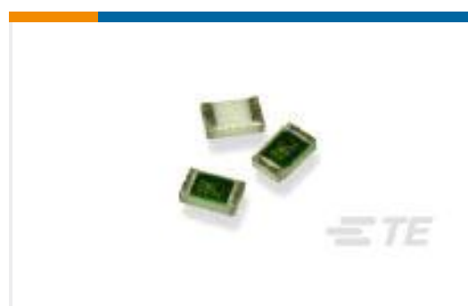
TE Part #2-1879212-0 CPF 0402 33K2 0.1% 25PPM 5K RL
