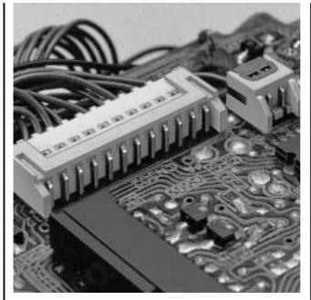
The KR connector features a mounting height as low as 6.9mm (.272") and a thickness as thin as 4.8mm (.189") (for top entry type). It is suitable for interconnection of a wide range of electronic equipment such as VCRs, video cameras, car stereo systems and communication equipment.
