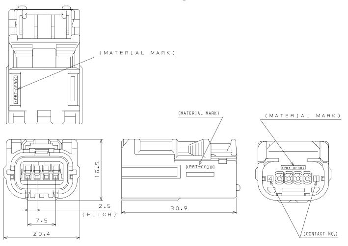
For 2pos. (MX36002SQ3) only the rear cover(shape, color) will be different (SJ Drawing SJ101632)
