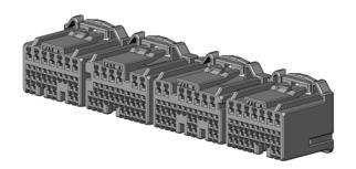
High density and non-water proof type of MX31 series is developed to meet the demands for compact and lighter connectors with multi pin counts, due to increase of computerized control in automotives. Pitch of signal terminal is 2.2mm, and the pitch of power terminal is 3.2mm. Compact and 4row type and the variation of the number of terminal is from 70pos. to 135pos. (pin header) This connector meets with automotive specs. and the application is for Automotive EUC (Engine, transmission, etc)
