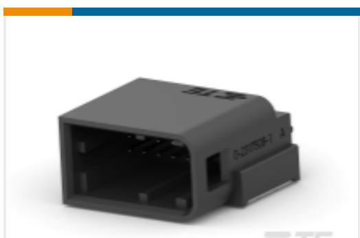
TE Part #2317507-1 2X6POS,NANOMQS,HDR ASSY, 90DEG,SMD,COD A
