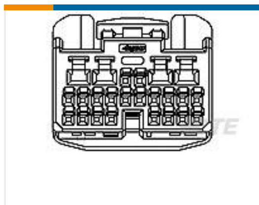
TE Part #1746864-1 0.64III/2.3II 24POS PLUG ASSY
