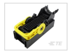
Connector & Housing Type: Housing for Female Terminals Mating Tab Width: 1.6 mm, 2.8 mm [ .063 in, .11 in ] Connector System: Wire-to-Board, Wire-to-Device, Wire-to-Wire Number of Positions: 62 Centerline (Pitch): 4 mm, 5 mm [ .157 in, .197 in ]
