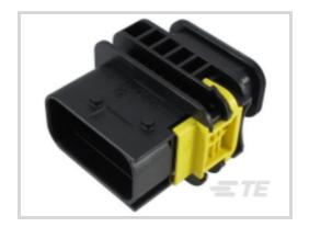
Connector & Housing Type: Housing for Male Terminals Mating Tab Width: 1.6 mm, 2.8 mm [ .063 in, .11 in ] Connector System: Wire-to-Wire Number of Positions: 10 Centerline (Pitch): 4 mm, 6 mm [ .157 in, .236 in ]
