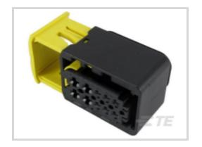
Connector & Housing Type: Housing for Female Terminals Mating Tab Width: 1.5 mm, 2.8 mm [ .059 in, .11 in ] Connector System: Wire-to-Wire Number of Positions: 10 Centerline (Pitch): 4 mm, 6 mm [ .157 in, .236 in ]
