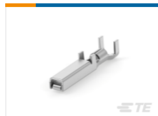
TE Part #917485-5 Contact: Component To Wire; 15A, 28-14 wire size
